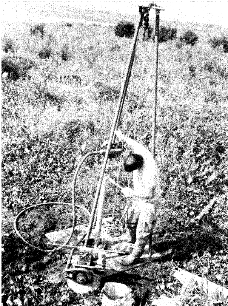
Figure 7-9. Photograph of a portable vibratory sampler (after Smith, Dunbar, and Britsch 1986). Note: Safety is a very important consideration for Corps of Engineers projects. Safety items, including hardhats, gloves, safety shoes, protective clothing, and dust or vapor masks, should be worn, as appropriate, for the particular drilling and sampling operation
